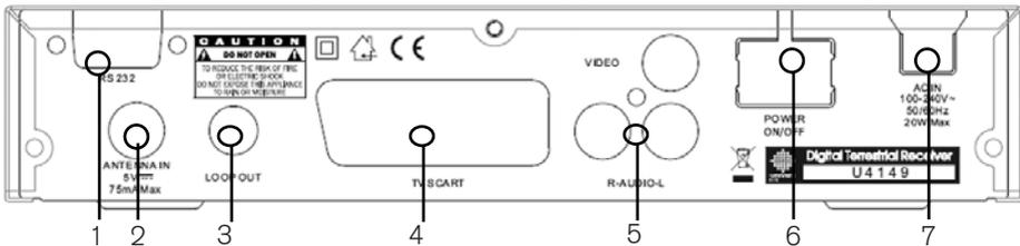
1. RS-232: Serial Port allowing software upgrades
